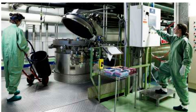
Staff at IRTA-CReSA using the digester, which disposes of the tissue samples and solid waste, ensuring that any microorganisms are totally deactivated.
